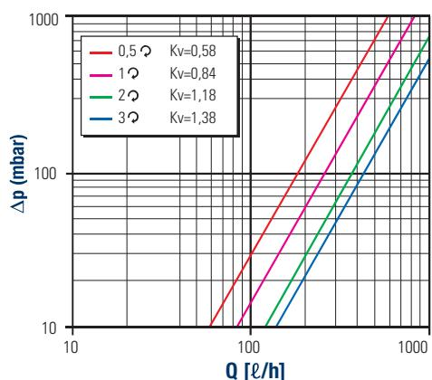
Pressure drop: 3/8" and 1/2" thermostatizable straight valve
